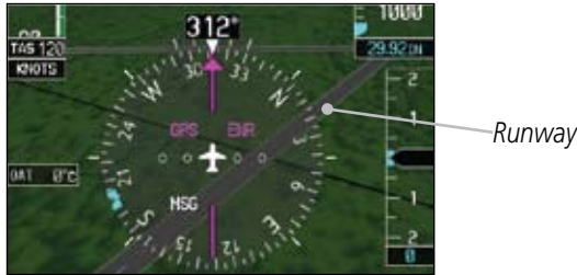
Figure 5-39 Depiction of Runway with a Loaded Flightplan
